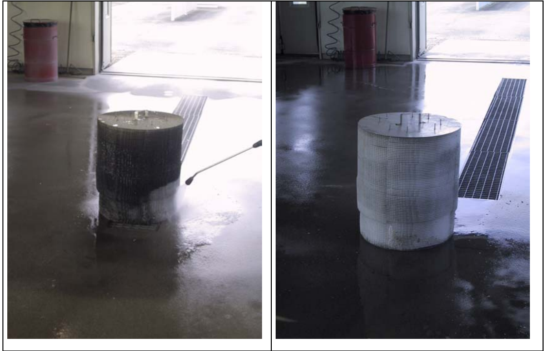
Figure 7. Cleaning of the coalescing unit by a high pressure washer and the coalescing unit after cleaning.
